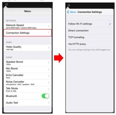
A user may choose connection types from <Follow setting for Wi-Fi>, <Direct connection>, <TCP tunneling> or <via HTTP proxy>.
